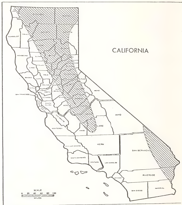
Figure 1.--Seismic risk zones in California (after Reference 1). The hatched area represents zone 2 and the remainder of the state, zone 3. The heavy black lines divide the state into northern, middle, and southern California as used in this report.
